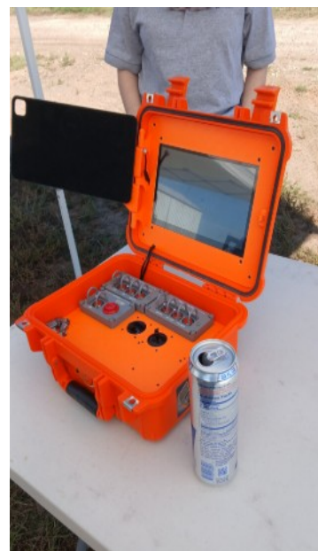
TECH IN THE FIELD - Zac Twigg's ground station with built in windows for his fluctus base station and a ipad pro mount that does a live feed from his "smarter rockets."
