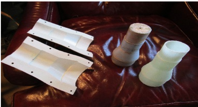
Illustration 4: Steve made these molds to produce the transition for his model
